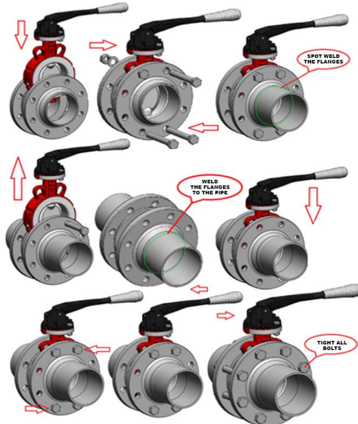
Fig. 6: Installing the valve between the flanges using screws
