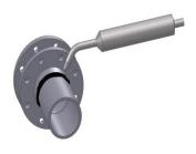
5. Weld the flanges to the piping.
