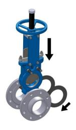
1. Position the gate valve with screw studs together with gaskets between the flanges.
