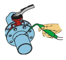
3. Attach the flanges at several points to the piping using a welding electrode.
