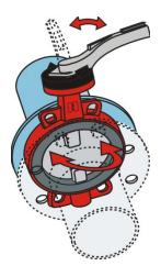
10. Test the proper function of the valve (the butterfly must not strike the piping).
