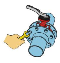
9. Add the remaining bolts and tighten them firmly (in a "crisscross pattern").
