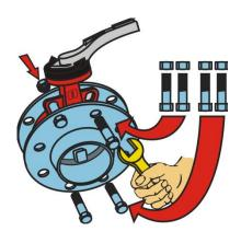
2. Lightly tighten the flanges with four bolts and align the position of the valve.
