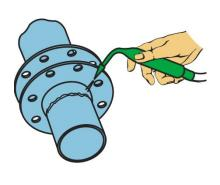
5. Weld the flanges to the piping.
