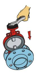
1. Place the valve with a slightly open butterfly between the flanges. The distance between the flanges is to be sufficient in order to prevent a damage to the seat.
