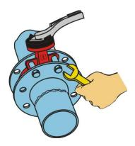
7. Align the valve and lightly tighten the valve using four bolts.
