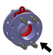
2. Tighten the flanges lightly with four bolts and align the position of the valve.
