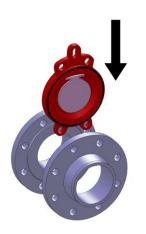
1. Place the valve between the flanges with sufficient distance between them.
