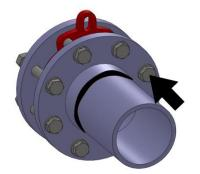
7. Centre the valve and tighten it lightly using four bolts. Add the remaining bolts (tighten them in a "criss-cross pattern").
