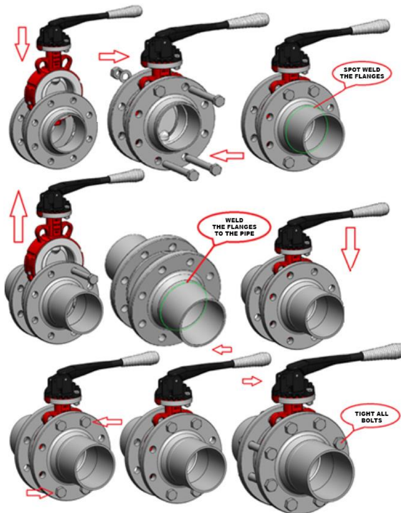
Fig. 6: Installing the valve between the flanges using screw
