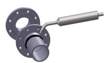
5. Weld the flanges to the piping.
