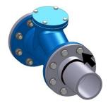
7. Centre the ball valve and tighten it lightly using four bolts. Add the remaining bolts (tighten them in a "criss-cross pattern").
