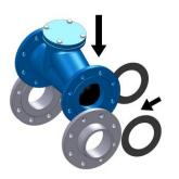
1. Position the ball valve between the flanges together with gaskets.
