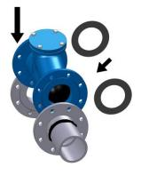
6. When the flanges have cooled down, insert the ball valve again with gaskets. The arrow on the body must coincide with the flow direction.
